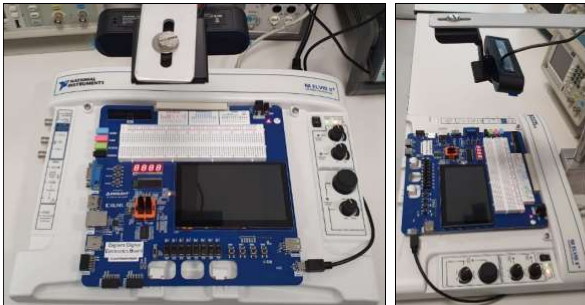
Figure 2: Front (left) and side (right) facing photos of the NI ELVIS II and Digilent Digital Electronics Board with mounted camera setup
