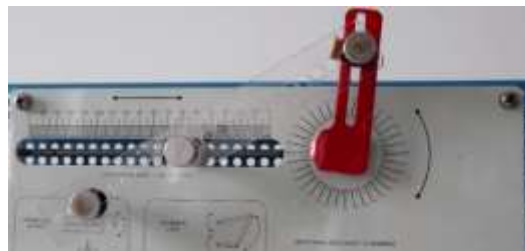
Figure 4: Three bar linkage - crank connecting mechanism
